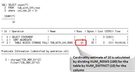
Figure 2. Cardinality calculation using basic table and column statistics
